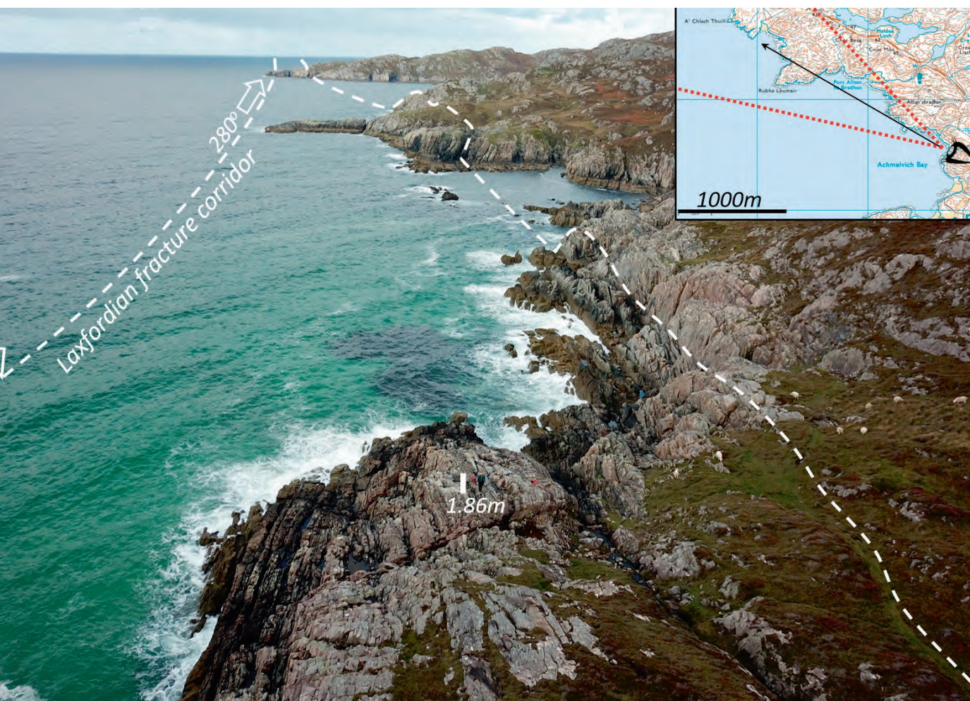
Annotated aerial photo of the north side of Achmelvich Bay. Taken with a DJI Mavic pro UAV. Annotations show the trace of the largest of the mapped fracture corridors in the Laxfordian brittle shear zone
